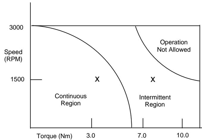
Fig.4.2 Speed-Torque Curve of a DC Motor
